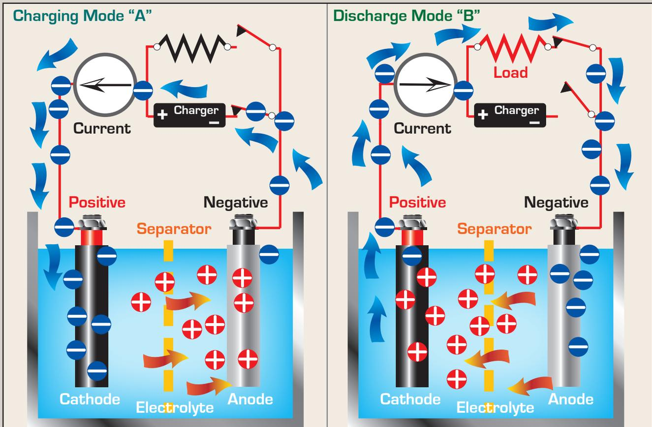
Negative ion and positive electron flow in charge mode "A" and discharge mode "B"
